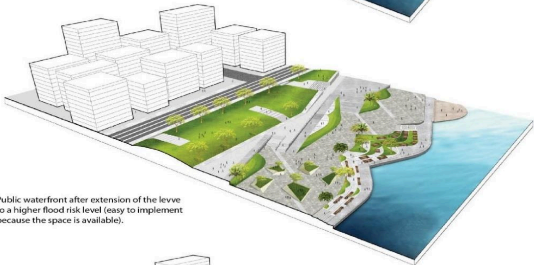
Creating public waterfront as placeholder for keeping the floodplain free and having space for enforcement of the embankment
